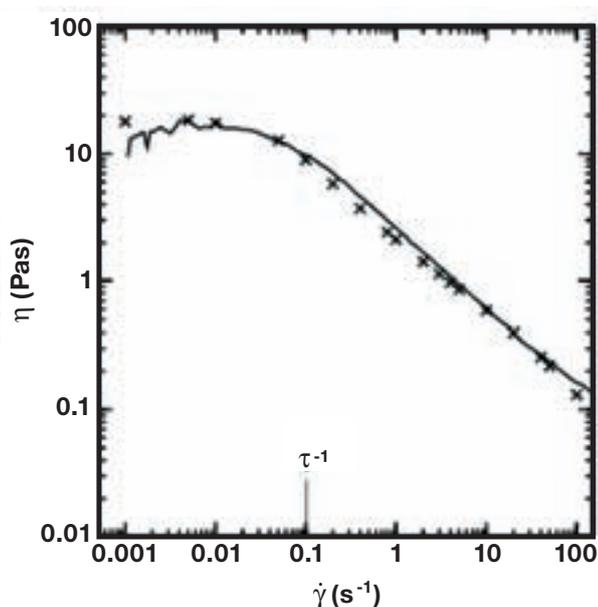
Viscosity versus shear rate for a synthetic resin. The line drawn is from experiments performed at Akzo-Nobel, Arnhem. Symbols are from simulations.
