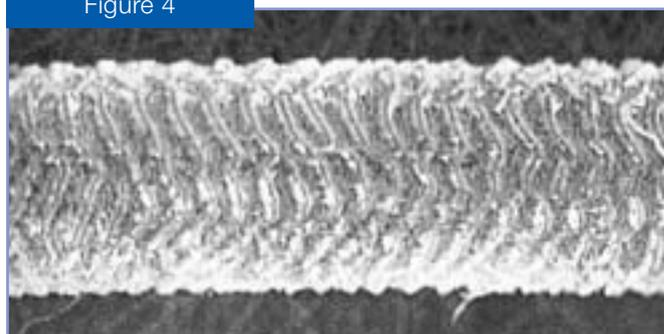
Micrograph of the sharkskin effect on an extruded polymer. From: J. Rheol. 45, 565 (2001)
